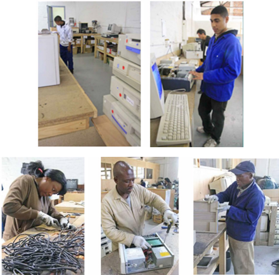
Figure 16: Dismantling, testing, repair and refurbishment
