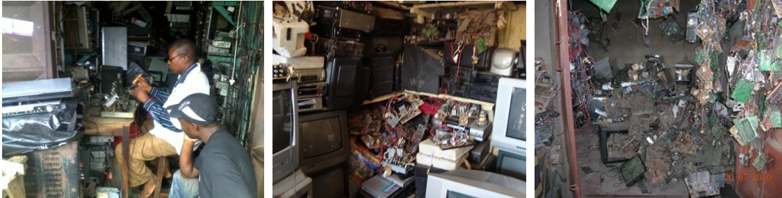
Figure 6.13: Refurbisher/repairers shops. (a) a refurbisher/repairer at work (b) un-repairable electronics are abandoned in a refurbishers shop (c) PWB recovered from un-repairable EEs displayed for sale. (Field survey Lagos, Aba and Kano)
