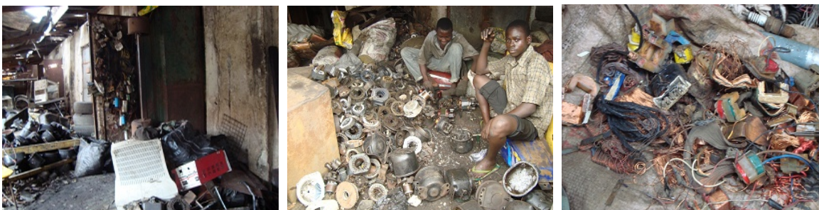
Figure 6.14: Material recovery from e-scrap (a) a recycler's shop (b) material recovery in progress; (c) recovered materials: copper wires.
