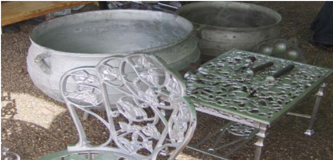
Figure 6.16: Recyclers display of products cast from compressor of refrigerators for local pots (Ikoko Irin) and other furniture
