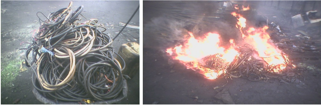
Figure 6.15: Open burning of waste cables to recover metals
