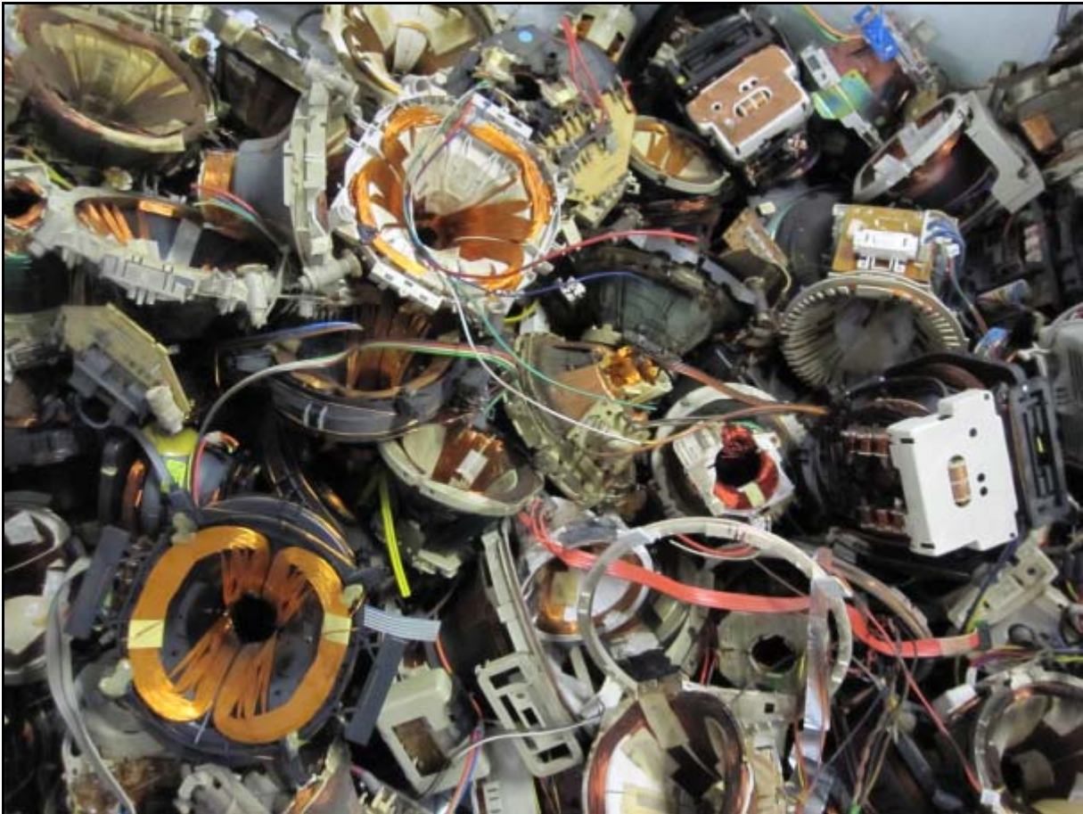
Photo 9 Focusing and deflecting coils of manually dismantled CRTs (Source: Öko-Institut 2010)
