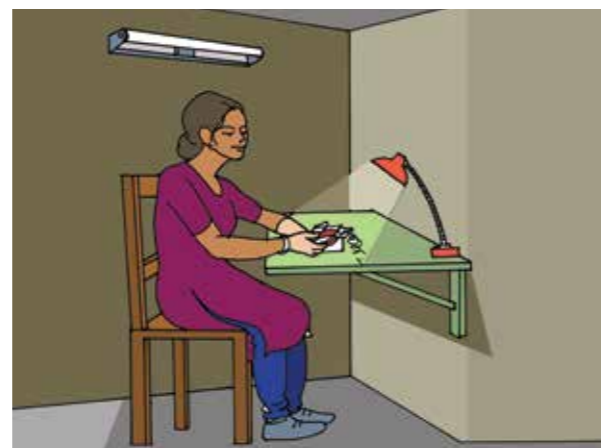
Figure 19. Use local task lights to ensure sufficient brightness necessary for work.
