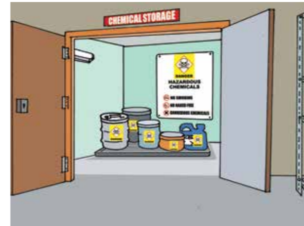
Figure 20. Store hazardous chemicals outside work areas with a firm lock.
